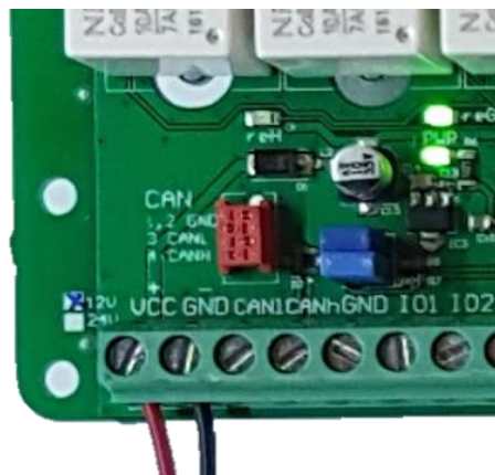
Figure 1: CAN bus connector (red)
