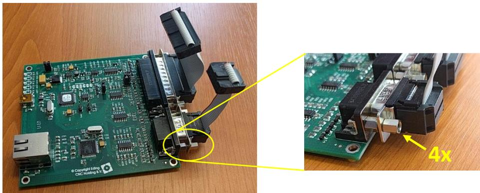
**Step 4. Mount CPU5A3/CPU5A4/CPU5A4E**
